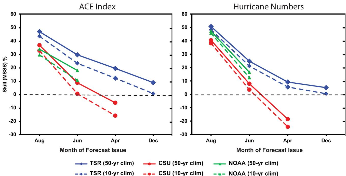
Forecast precision is assessed using the Mean Square Skill Score (MSSS) which is the percentage improvement in mean square error over a climatology forecast. Positive skill indicates that the model performs better than climatology, while a negative skill indicates that it performs worse than climatology. Two different climatologies are used: a fixed 50-year (1951-2000) climatology and a running prior 10-year climate norm.
